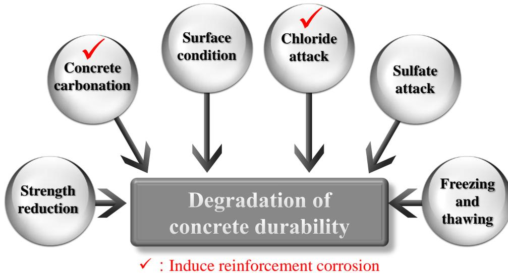
**Fig. 1** Combined deterioration factors affecting on durability of concrete
