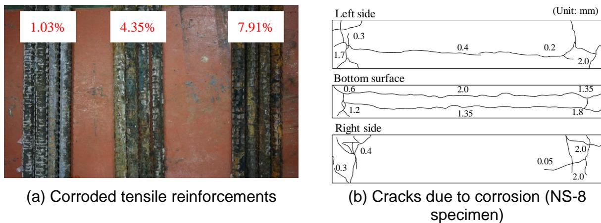
**Fig. 3** Accelerated corrosion test results
